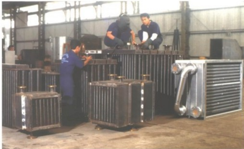
Thermal Oil to Air for Air Heater
